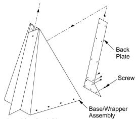
Figure 4 - Attaching Back Plate
